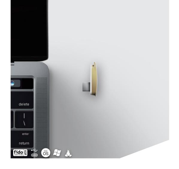
FIDO U2F certified security key with USB Type-C port and compact body which fits on a key-chain or mounted in a spare USB Type-C port on your PC.
