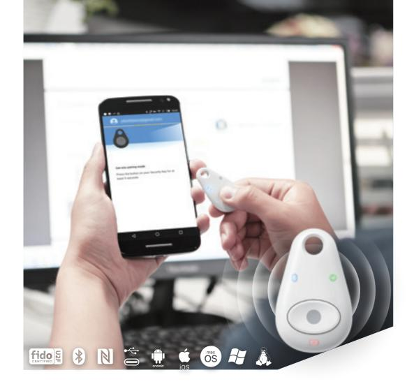
FIDO U2F certified security key which works on 3 different interfaces: USB Type-C / Micro USB, NFC, and Bluetooth.
